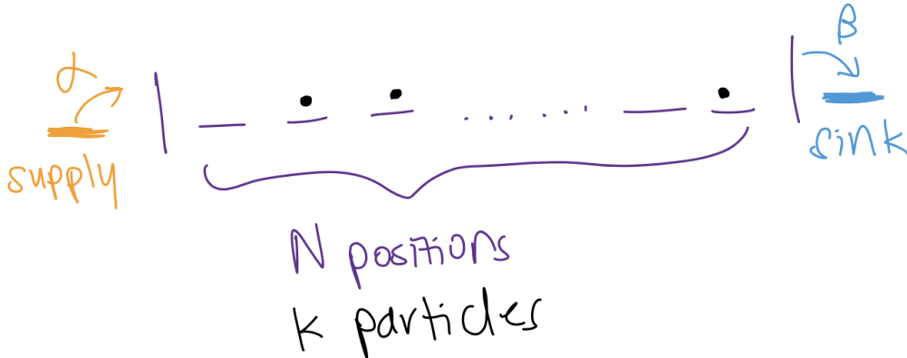
Figure 2: Illustration of the acyclic asymmetric process, as a linear chain (rather than a cyclic chain, as in the cyclic asymmetric process).
