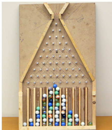
Figure 5: A Galton Board, a device invented to demonstrate the law of large numbers, in particular that with sufficient sample size the binomial distribution approximates a normal distribution.
